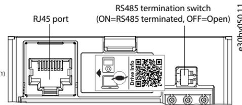
Illustration 4: RJ45 Port and RS485 Termination Switch
